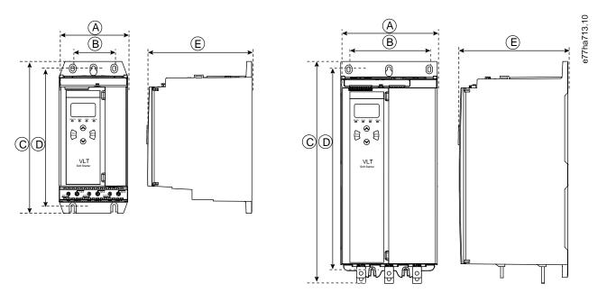
Illustration 3: Dimensions, Frame Sizes S1 (Left) and S2 (Right)
