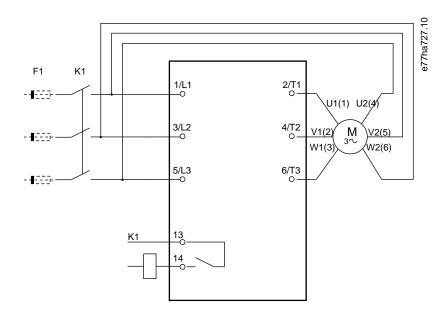
K1 Main contactor F1 Fuses or circuit breaker (optional  $^{\theta}$ )
