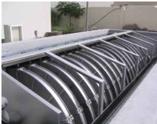
RoDisc® features filter discs arranged horizontally and rotate on central shafts powered by Bauer BF Series gear motors.
