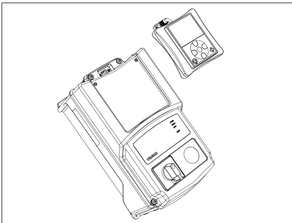
Figure 49. Mounting of the keypad.
