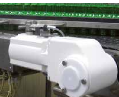
A cover is also provided for shaft ends used in gears for hygiene critical areas.
