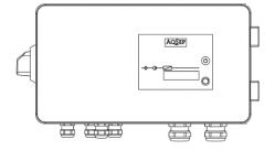
The control box is connected to the sensors on the hydraulic unit via a cable tree of 3 m (9.9 ft.). Separate cables connects the electrical motor and valve.
